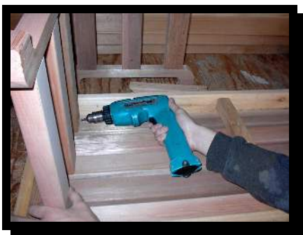
Attach prebuilt legs
